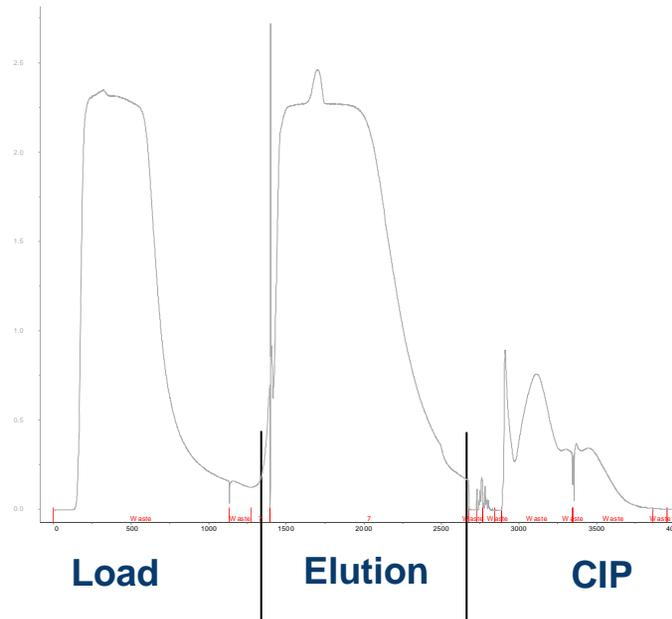
The minor differences in peak shape are attributable to equipment differences at the 15 mL and 500L scales, the composition of each of the fractions is comparable
