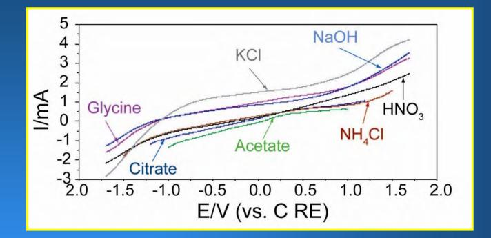
Linear Sweep Voltammetry scanned at 0.3 V/s. 0.1 M Electrolyte Concentration Glycine and Ammonium Chloride pH9 Sodium Hydroxide pH 12 Acetate Buffer pH 4.6 Citrate Buffer pH 2.5
