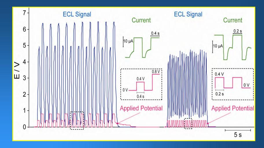
Time Course Step Potentials and the Corresponding ECL Response of the Luminol-H<sub>2</sub>O<sub>2</sub> System.
