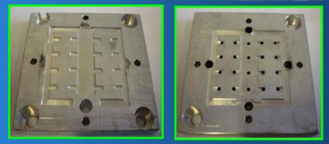
Mould Cavity for the Electrical Connectors
