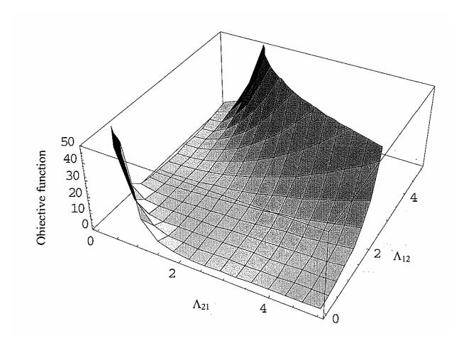
Variation of objective function with the two Wilson binary interaction parameters for the Ca – Na binary system.
