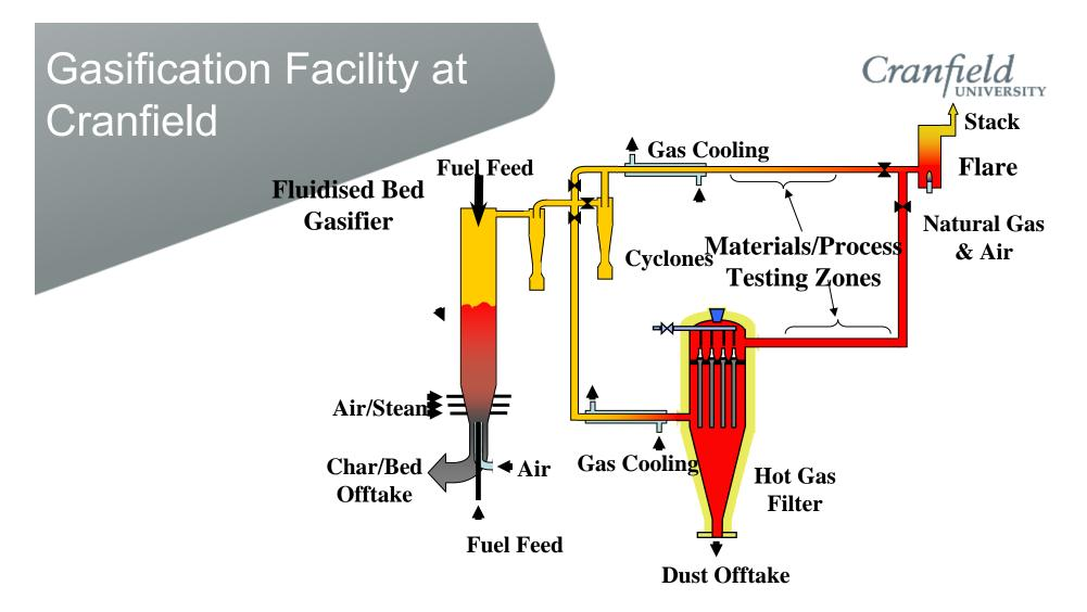
Spouted fluidised bed gasifier – 0.15m diameter In- and above-bed feed systems for all types of solid fuels (up to 15kg/h) and sorbents Fluidisation with air and/or steam
