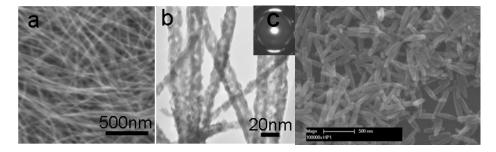
Figure 1. (a) Bundles of tungsten oxide nanowires synthesized by hydrothermal; (b) Tungsten nitride nanowires converted using the tungsten oxide bundles; and (c)  $Fe_2O_3$  nanorods synthesized by the hydrothermal process.
