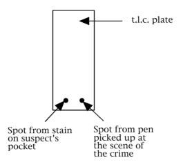
Carefully put the plate into the tank with the spots at the bottom and wait until the solvent has almost reached the top of the plate. This will take about 5 minutes.
