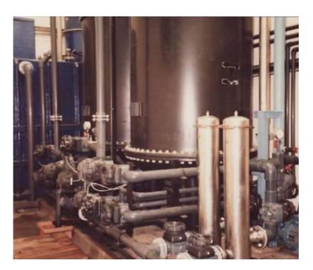
Larger vessels in rubber lined or PVC dipped carbon steel up to 3600mm dia
