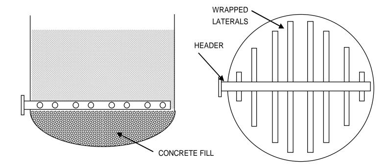
Concrete fill with wrapped laterals For custom engineered steel vessels > 1000mm diameter
