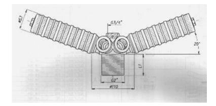
Hub and radial underdrain For vessels up to  $1000\phi$
