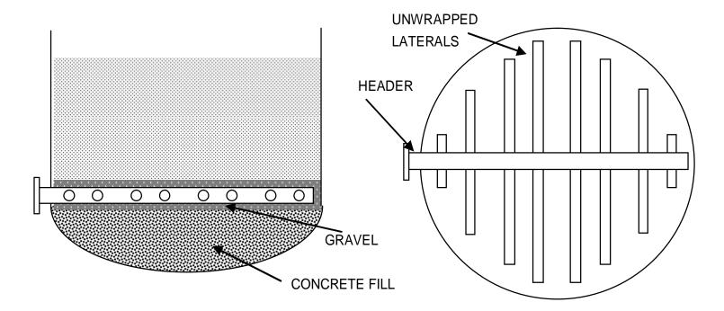
Concrete fill with unwrapped unwrapped laterals and gravel For custom engineered steel vessels > 1000mm diameter
