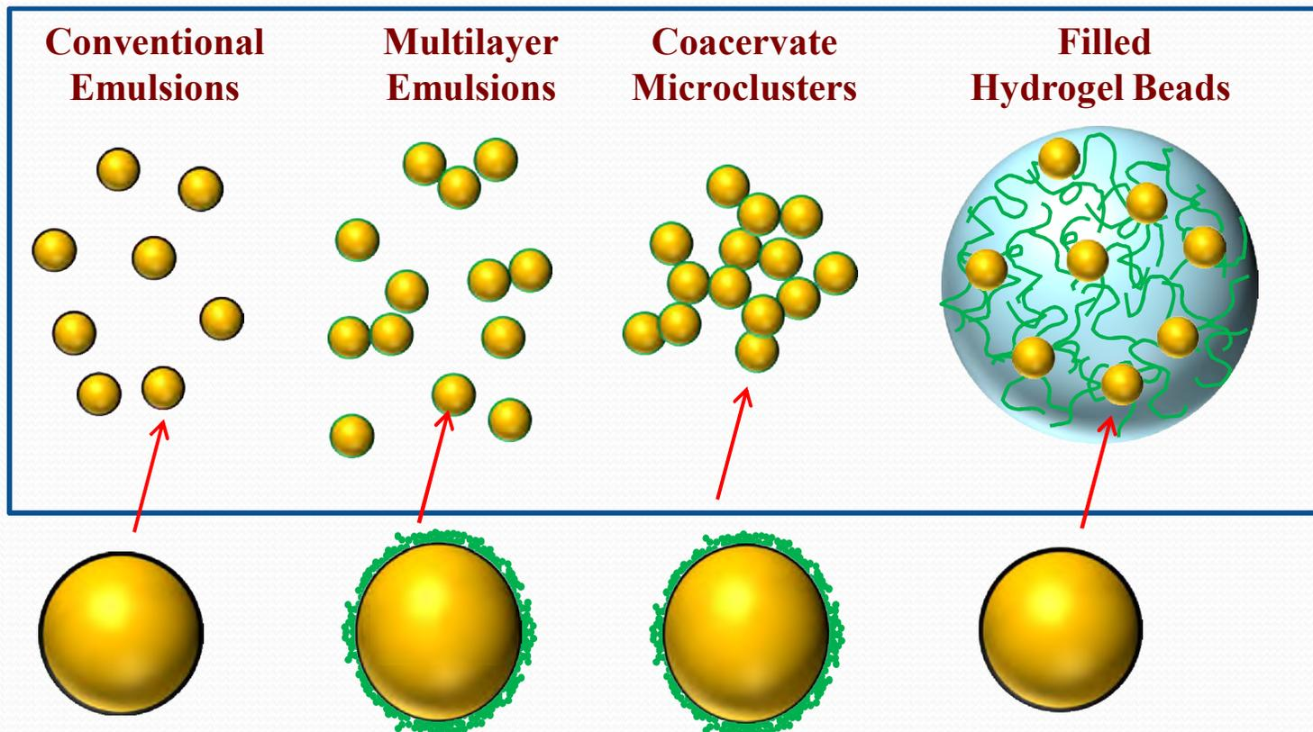
(A) conventional emulsion; (B) multilayer emulsion; (C) coacervate microclusters; (D) filled hydrogel beads fabricated from corn oil, whey protein, chitosan and/or alginate.
