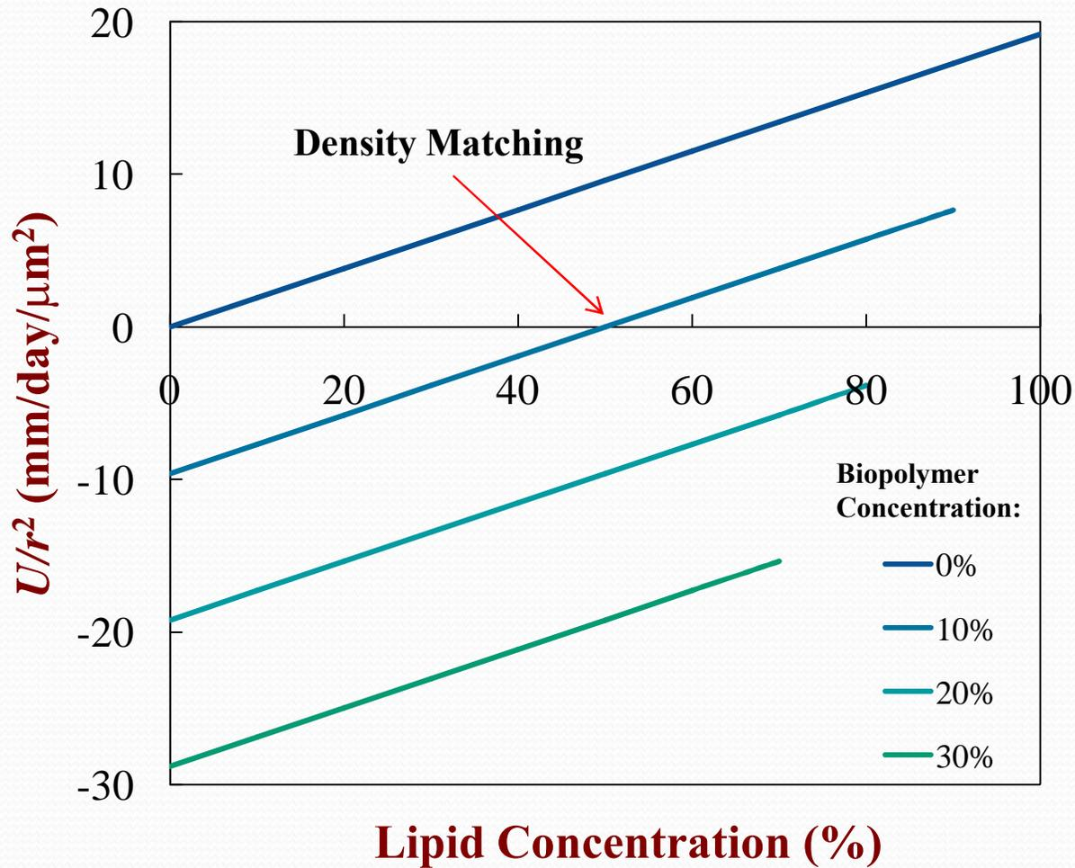
Theoretical prediction of the influence of biopolymer particle composition (lipid and biopolymer concentration) on the stability to gravitational separation. Assumed densities: biopolymer =  $1500 \text{ kg m}^{-3}$ ; water =  $1000 \text{ kg m}^{-3}$ ; oil =  $900 \text{ kg m}^{-3}$ .
