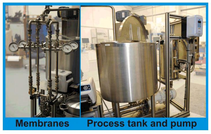
Four tube – insert system (100 kg/h)
