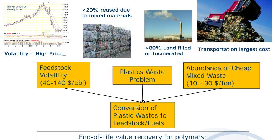
Polymer recovery > monomer recovery > feed stock recovery > incineration > landfill
