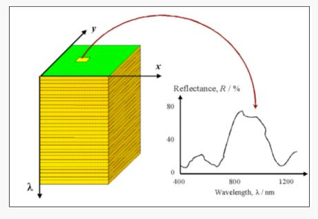
HSI emerging platform technology that integrates conventional computer vision and spectroscopy. It combines the advantages of both technologies by providing spatial, spectral, and multi-constituent information, while also being sensitive to minor constituents.
