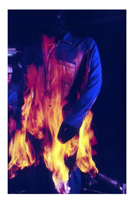
Instrumented Manikin (eg DuPont Thermoman ®) for Testing Protective Clothing Fire Performance:
