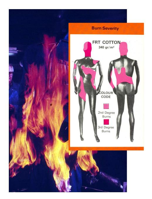
Instrumented Manikin (eg DuPon Thermoman ®) for Testing Protective Clothing Fire Performance:
