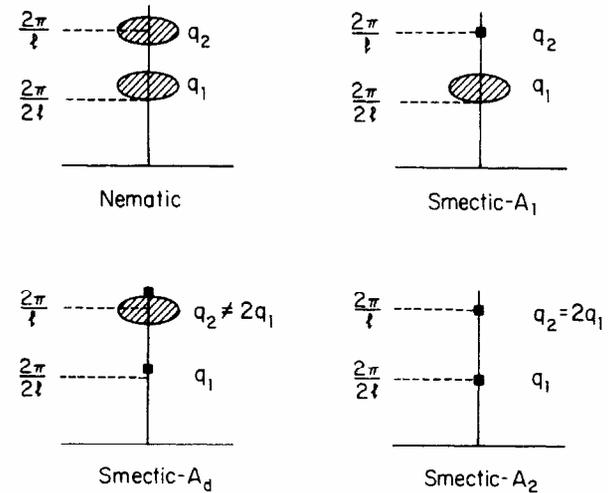
FIG. 2. Diffraction patterns of the polar nematic and smectic-A phases. The vertical axis indicates the  $q_z$  direction and the horizontal axis indicates the  $q_x q_y$  plane. The small solid squares denote Bragg-like spots and the large ellipses denote diffuse spots. The monolayer ordering ( $d = l$ ) produces the scattering at  $q_2$  and the dipolar ordering ( $l < d \leq 2l$ ) produces the scattering at  $q_1$ .
