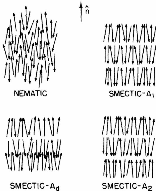
FIG. 1. Schematic representation of the polar nematic and smectic-A phases. The molecules are drawn as thin rods with an arrow on one end to denote the lack of inversion symmetry produced by an off-center dipole.
