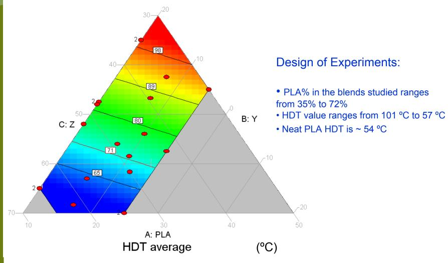
Testing Methods: Deflection Temperature Under Flexural 66 psi Load: ASTM D648
