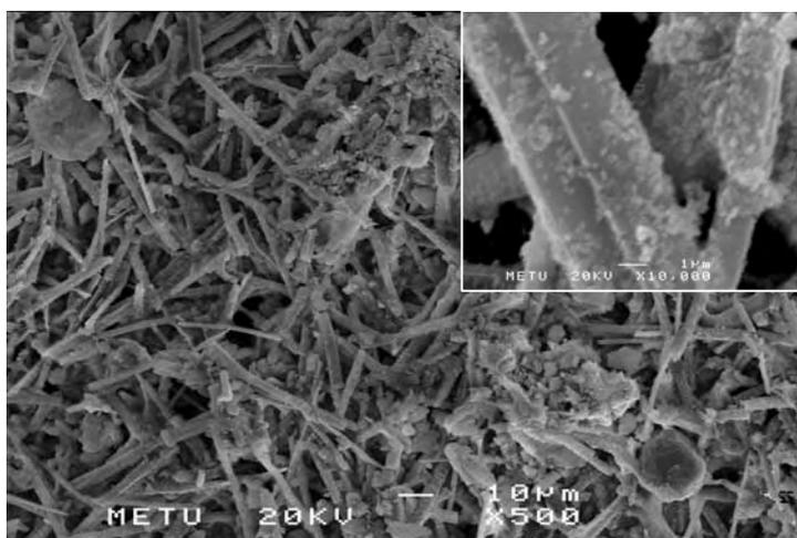
Figure 1. SEM image of HA/chitosan nanocomposite prepared at mass ratio of 80-20 %
