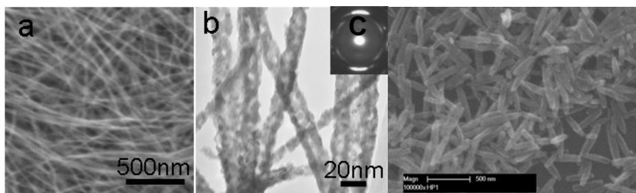
Figure 1. (a) Bundles of tungsten oxide nanowires synthesized by hydrothermal; (b) Tungsten nitride nanowires converted using the tungsten oxide bundles; and (c)  $\text{Fe}_2\text{O}_3$  nanorods synthesized by the hydrothermal process.
