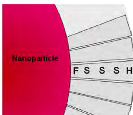
Schematic representation of a ligand shell coating and protecting a nanoparticle from the surrounding environment.
