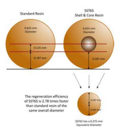
Why is SST resin so Efficient in Cyclic Ion Exchange?
