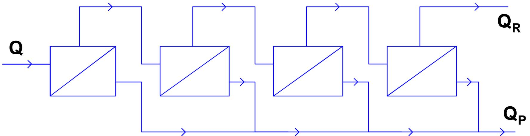
$$Q_R = Q (1-\theta)^n, \text{ where } \theta = \text{conversion per element and } n = \text{no. elements}$$
