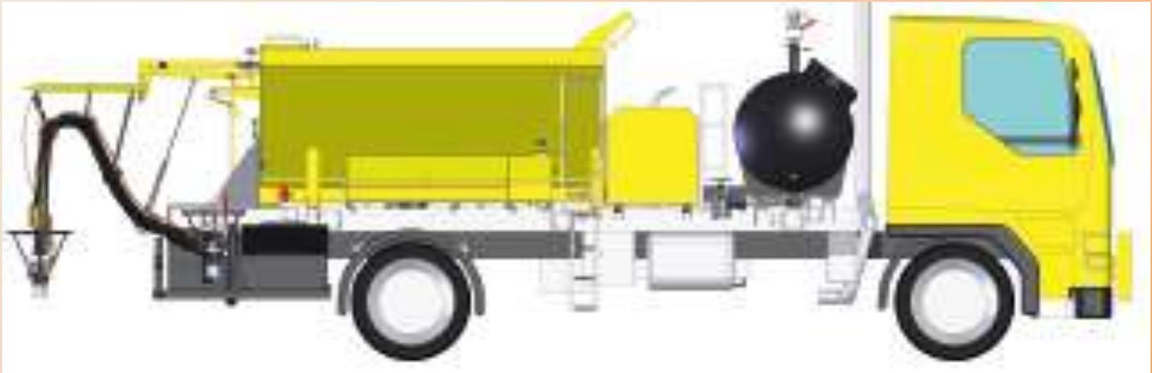
**Self contained, 2 man operation – Repairs c.200 Potholes before refilling**
