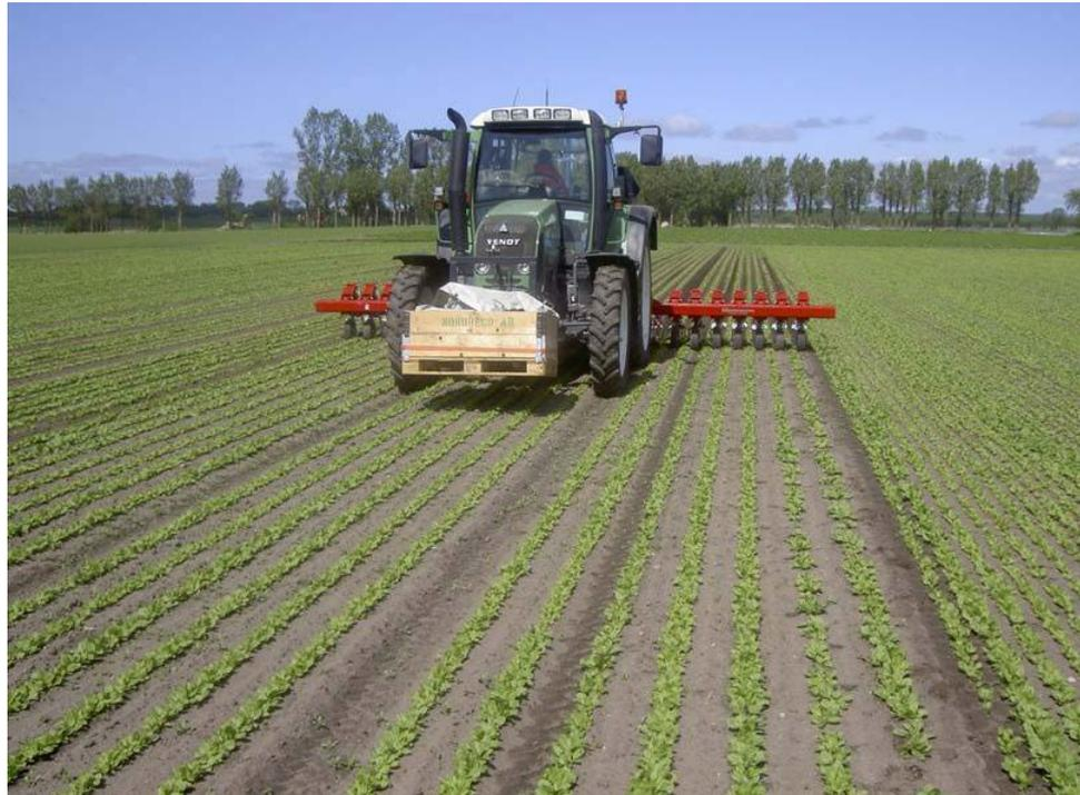
**With the ability to accurately and repeatably place seed, fertiliser and agrochemicals Active Implement Steer will cause a revolution in crop seeding, fertilising and agrochemical application in the next decade.**
