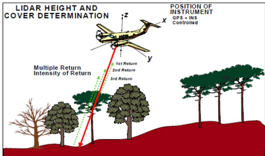
In this example, the first return measurement is a range value of the tree top; the last return is the ground. Lidar systems can return up to four range values and three intensity values for ground and above-ground elevation data from a single flight.
