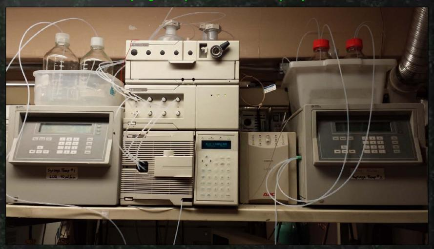
50 mM NH<sub>4</sub>OCOH @ 40  $\mu$ L/min for ESI-MS + D.I. H<sub>2</sub>O for source wash between runs
