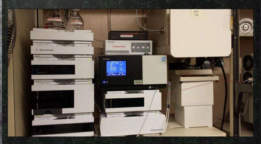
Quaternary Pump/Autosampler/Column Thermostat/UV Detector/Corona CAD/ELSD
