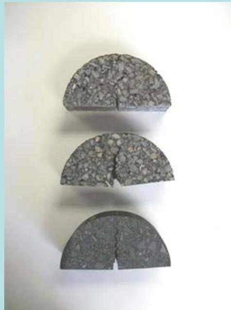
**Semi Circular Bending Test**
