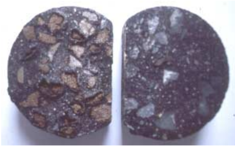
Figure 7 HRA samples containing unsound and sound basalt after five magnesium sulphate soundness cycles
