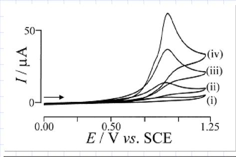
Cyclic voltammograms (scan rate 0.02 V s<sup>-1</sup>) for the oxidation of 1 mM hydrogen peroxide in the presence of (i) 0.1 mM, (ii) 0.4 mM, (iii) 1.0 mM, and (iv) 2.0 mM KOH in aqueous 1.0 M KNO<sub>3</sub> at a boron-doped diamond electrode (0.25 cm<sup>2</sup>) modified with hydrous ferric oxide.
