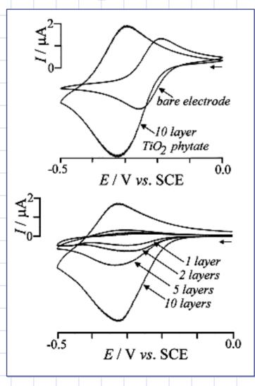
Reversible one electron process  $Ru(NH_3)_6^{3+}(aq) + e^{-1}$  $\rightarrow \text{Ru(NH}_3)_6^{2+}(aq)$ New voltammetric response at  $E_{p}^{red} =$ -0.33 V vs. SCE Adsorption of  $Ru(NH_3)_{6}^{3+}$  into TiO<sub>2</sub> phytate film
