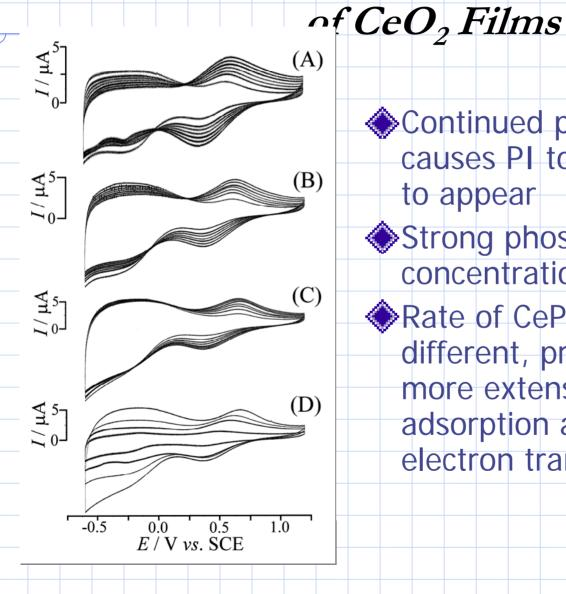
Continued potential cycling causes PI to diminish and PII to appear Strong phosphate concentration effect ◆Rate of CePO₄ formation is different, presumably due to more extensive phosphate adsorption and better electron transport
