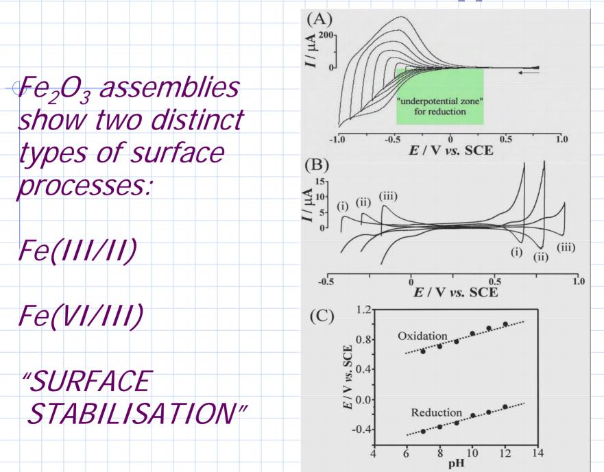
Nanoparticle Thin Film Voltammetry IV.: Reactivity of Fe<sub>2</sub>O<sub>3</sub> Assemblies
