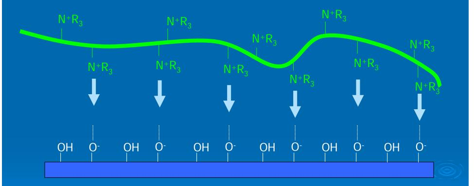
Ionic adsorption of Zetag on to a glass surface is achieved via (O<sup>-</sup> N<sup>+</sup>R<sub>3</sub>) ion-pairs
