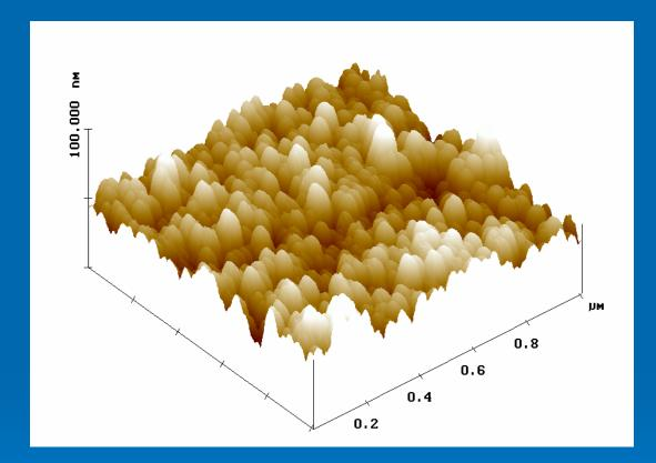
21 nm Silica particles attached to glass substrate
