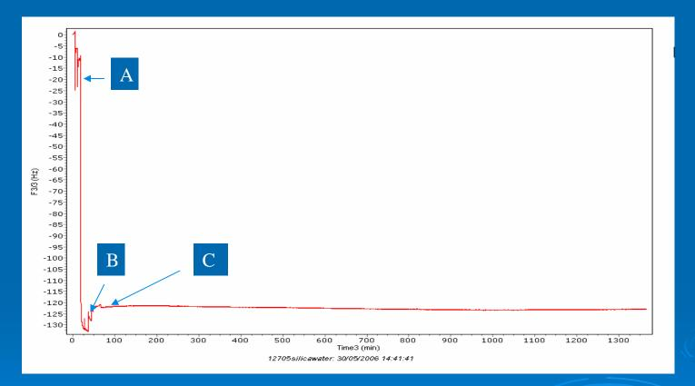
A :deposition of Zetag<sup>™</sup> and 7nm silica coating
