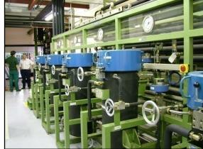
**Production-scale** supercritical CO2 extractor
