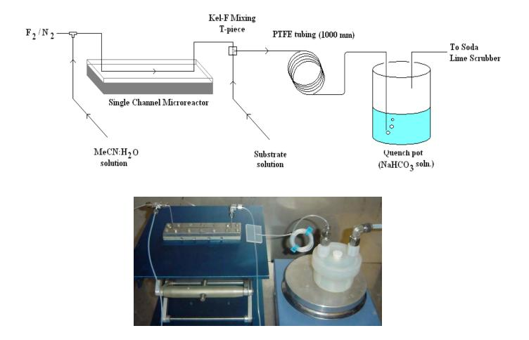
Applicable to large scale synthesis using continuous flow techniques
