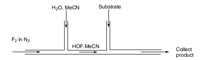
Gas/liquid - liquid/liquid sequential flow reaction
