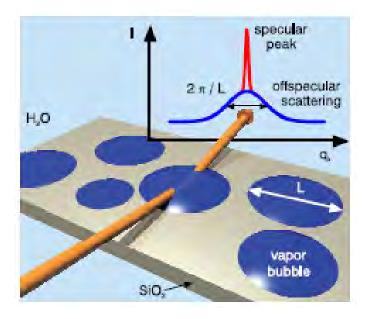
Sketch of the scattering in forward direction from an interface Covered by randomly spaced bubbles
