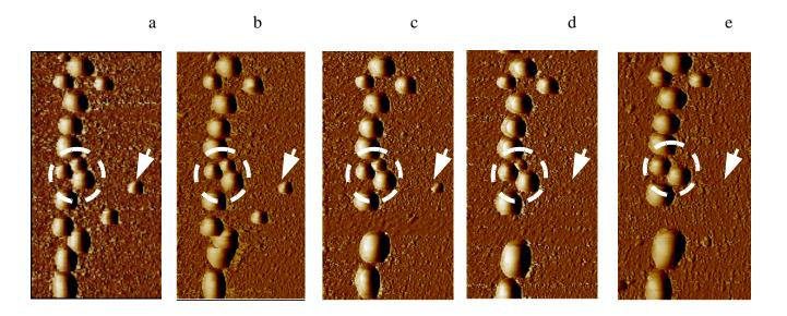
TMAFM bubble coalescence images: (a) made at 20 hours after CO<sub>2</sub> saturated water was injected into the fluid cell. (b), (c), (d) and (e) made at time intervals of 20 minutes after (a).Scan Area:  $10 \,\mu\text{m} \times 5 \,\mu\text{m}$ , Height= 300nm. Phase images
