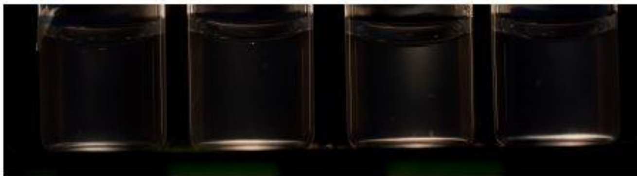
(a) Volume fractions of Beidellite are a) \phi_{\text{clay}} = 0.33\% ; b) \phi_{\text{clay}} = 0.35\% ; c) \phi_{\text{clay}} = 0.37\% ; and d) \phi_s = 0.39\%
