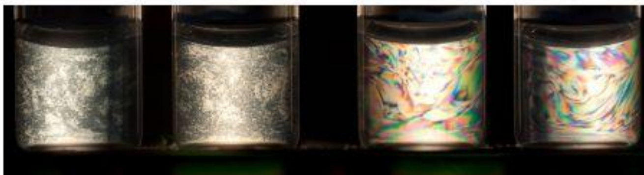
(c) Volume fractions of Beidellite are a) \phi_{\text{clay}} = 0.47\% ; b) \phi_{\text{clay}} = 0.48\% ; c) \phi_{\text{clay}} = 0.50\% ; and d) \phi_s = 0.51\%
