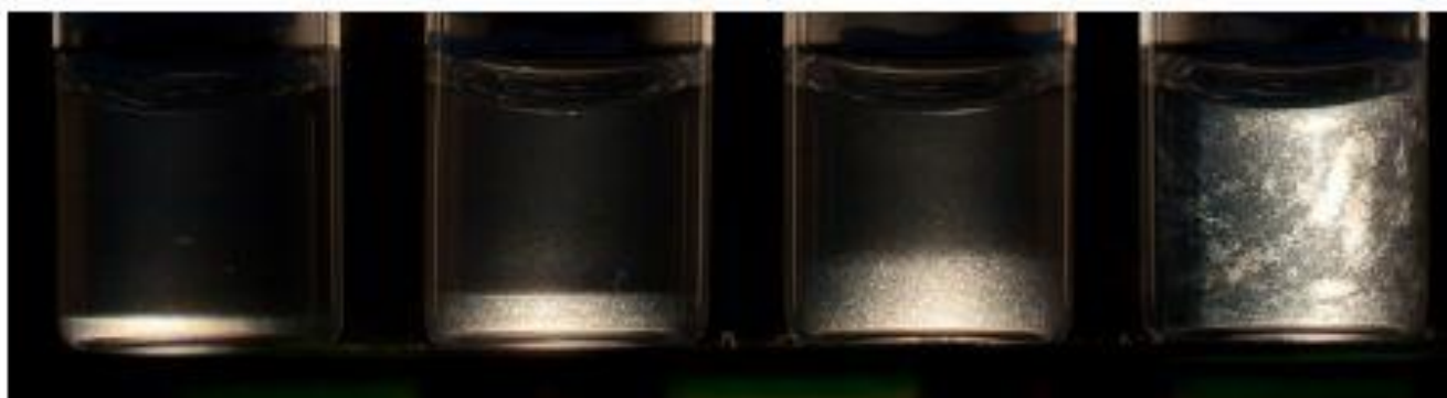
(b) Volume fractions of Beidellite are a) \phi_{\text{clay}} = 0.41\% ; b) \phi_{\text{clay}} = 0.42\% ; c) \phi_{\text{clay}} = 0.44\% ; and d) \phi_s = 0.46\% .
