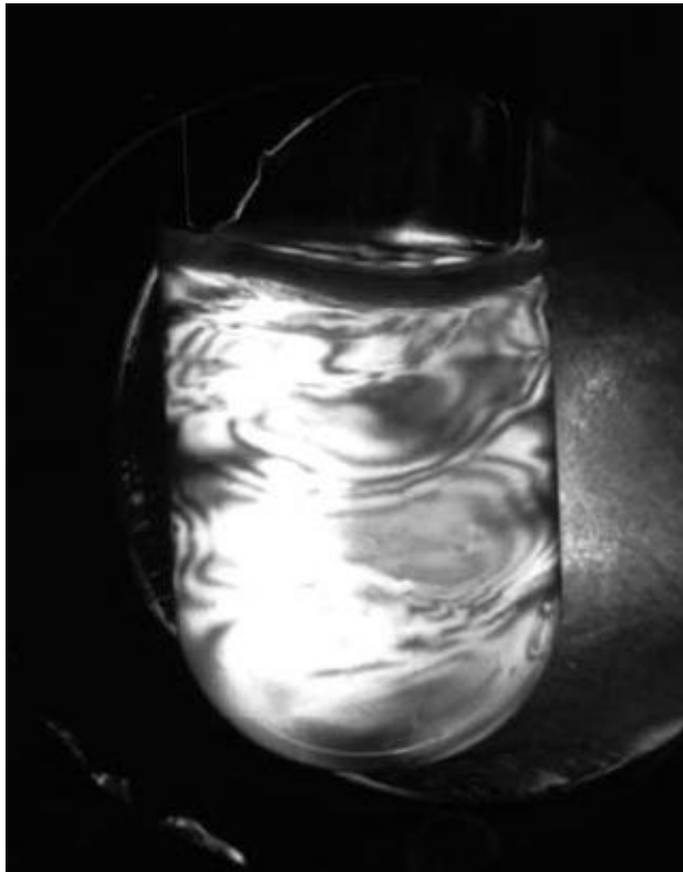
Bentonite suspension (4.3wt%) between cross polarizers
