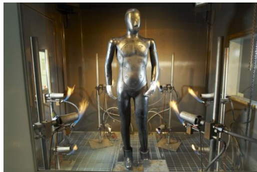
Instrumented manikin: ASTM F 1930 and BS EN ISO 469:2005 Annex E (method BS ISO 13506)
