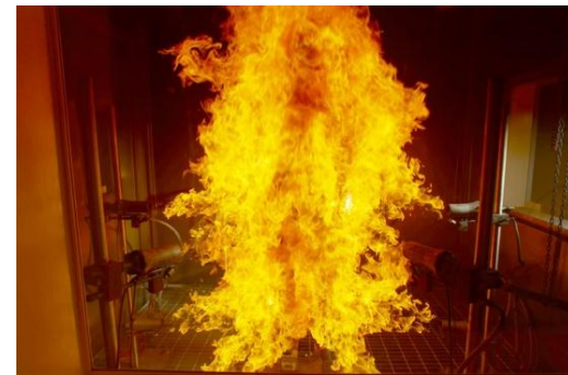
Instrumented manikin: ASTM F 1930 and BS EN ISO 469:2005 Annex E (method BS ISO 13506)
