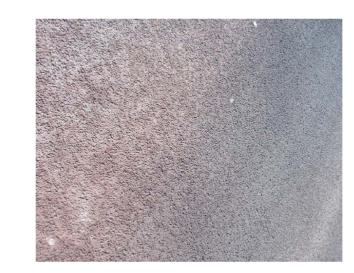
Red Asphalt: rapid colour fade under trafficking. Colour difference from load to load.
