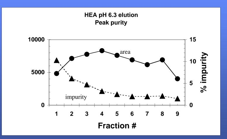
A less clean SP eluant was adsorbed onto HEA in 1 M ammonium sulfate, pH 8, washed with the same buffer without ammonium sulfate & eluted at pH 6.3. Individual fractions were assayed by RP HPLC
