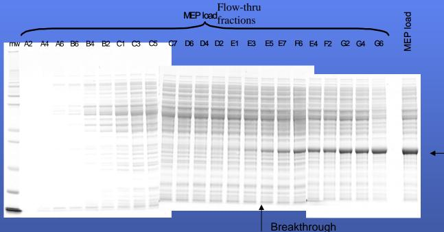
22.5 x 1.6 MEP column (45 ml)1.5 liters @2.9 g/liter loaded before breakthroughCapacity: ~98 mg target protein/ml MEP
