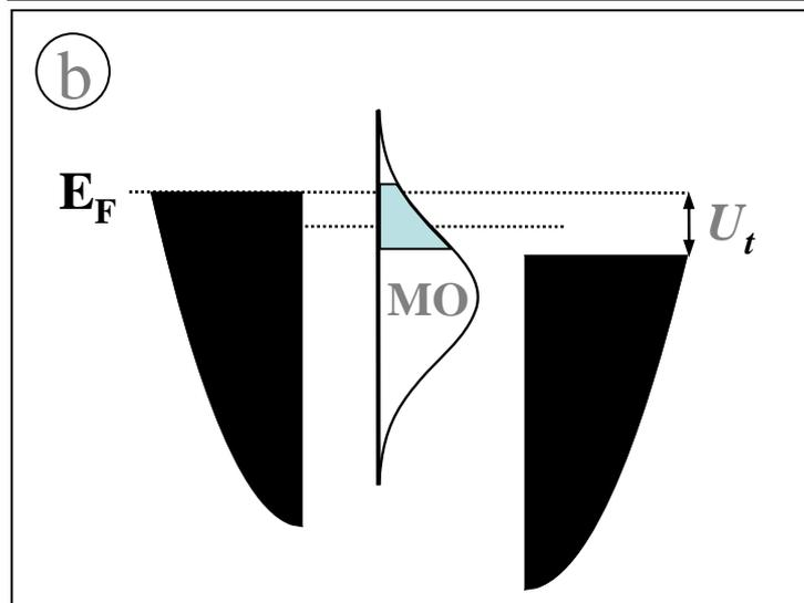
Build in functionality that has an orbital closer to Au Fermi level.
