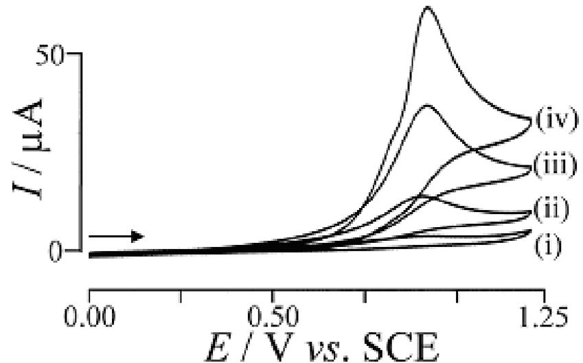
Cyclic voltammograms (scan rate 0.02 V s<sup>-1</sup>) for the oxidation of 1 mM hydrogen peroxide in the presence of (i) 0.1 mM, (ii) 0.4 mM, (iii) 1.0 mM, and (iv) 2.0 mM KOH in aqueous 1.0 M KNO<sub>3</sub> at a boron-doped diamond electrode (0.25 cm<sup>2</sup>) modified with hydrous ferric oxide.
