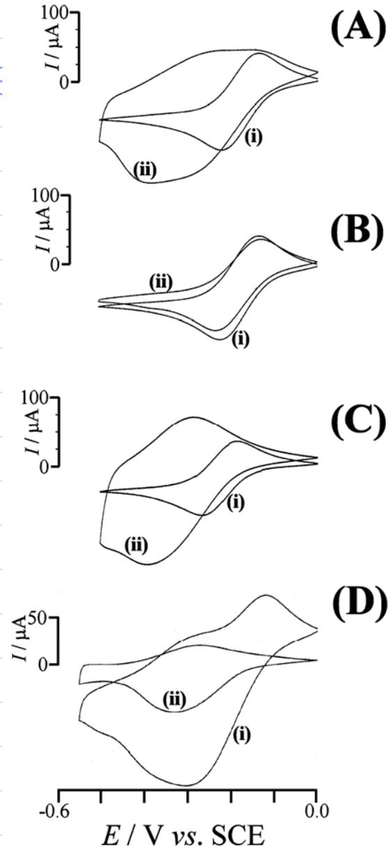
(A)  $\text{Ru}(\text{NH}_3)_6^{3+}$  on  $500^\circ\text{C}$  Calcined  $\text{TiO}_2$  Films
