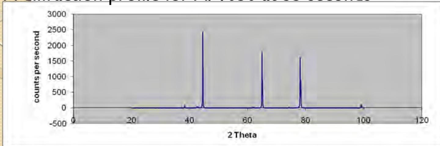
A diffraction profile for Al 6061 at 25 seconds
