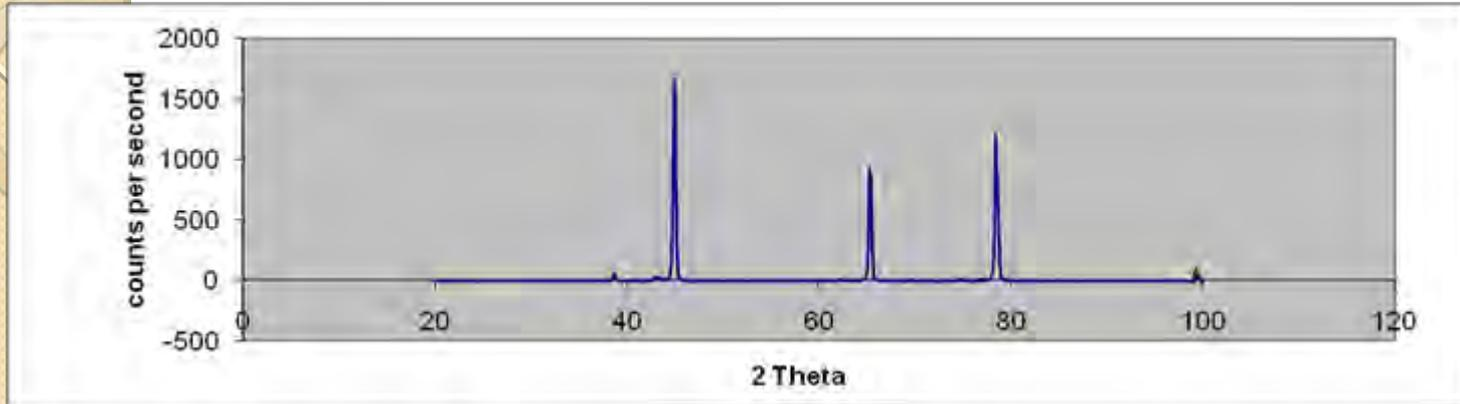
A diffraction profile for Al 6061 at 35 seconds
