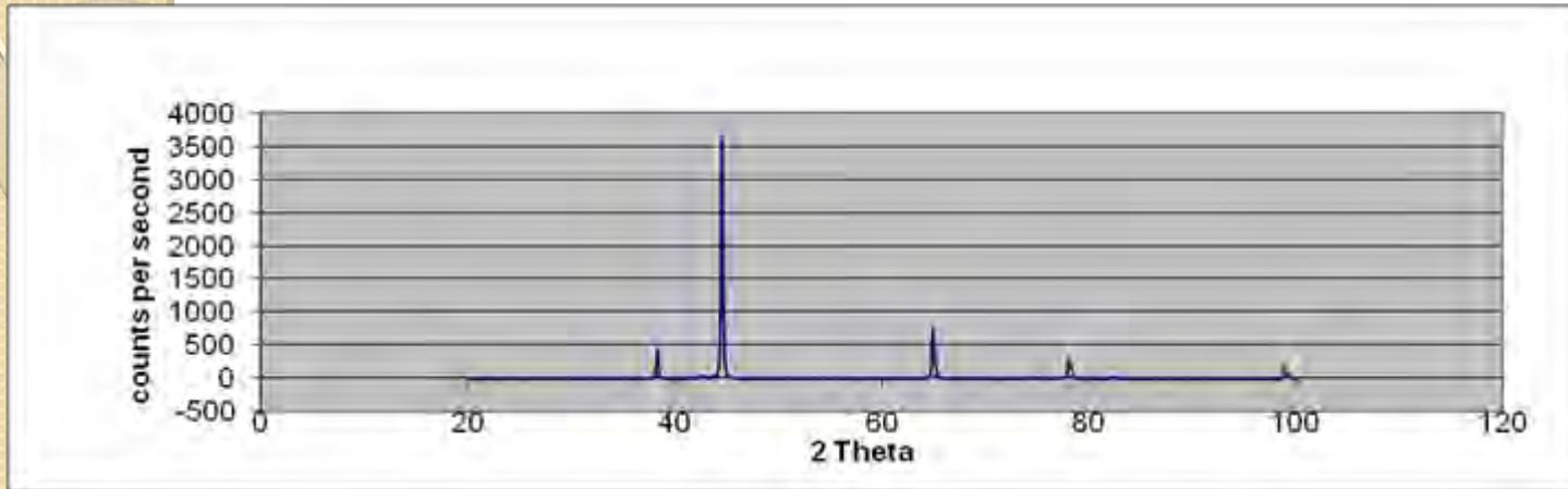
A diffraction profile for Al 6082 at 30 seconds
