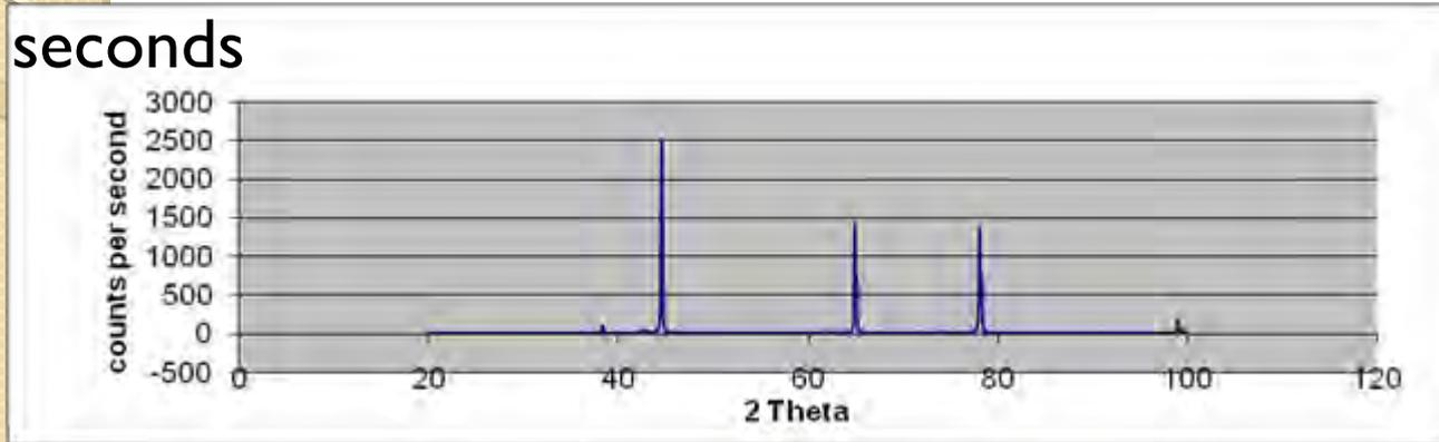
A diffraction profile for Al 1050 at 30 seconds
