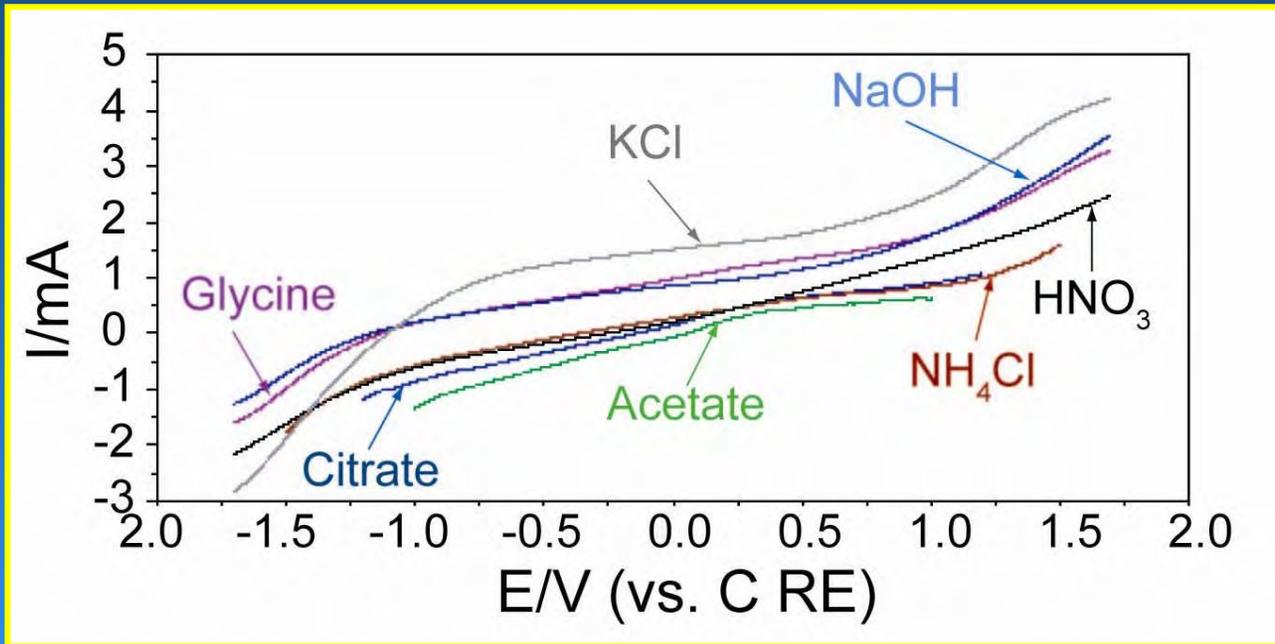
Linear Sweep Voltammetry scanned at 0.3 V/s.
