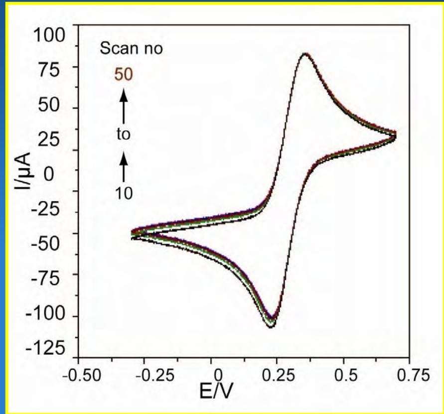
$3 \times 10^{-3}$  M Potassium Ferricyanide in 0.1 M KCl (vs. Ag/AgCl RE).
