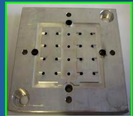
Mould Cavity for the Electrical Connectors
