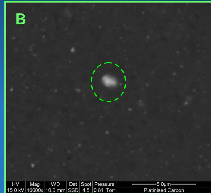
**SEM Images of A) Carbon, and B) Platinised Carbon Inks**
