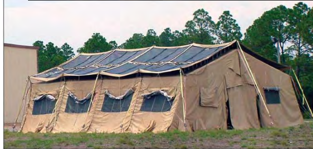
Figure 2. Flexible solar cell technology incorporated into a military tent
