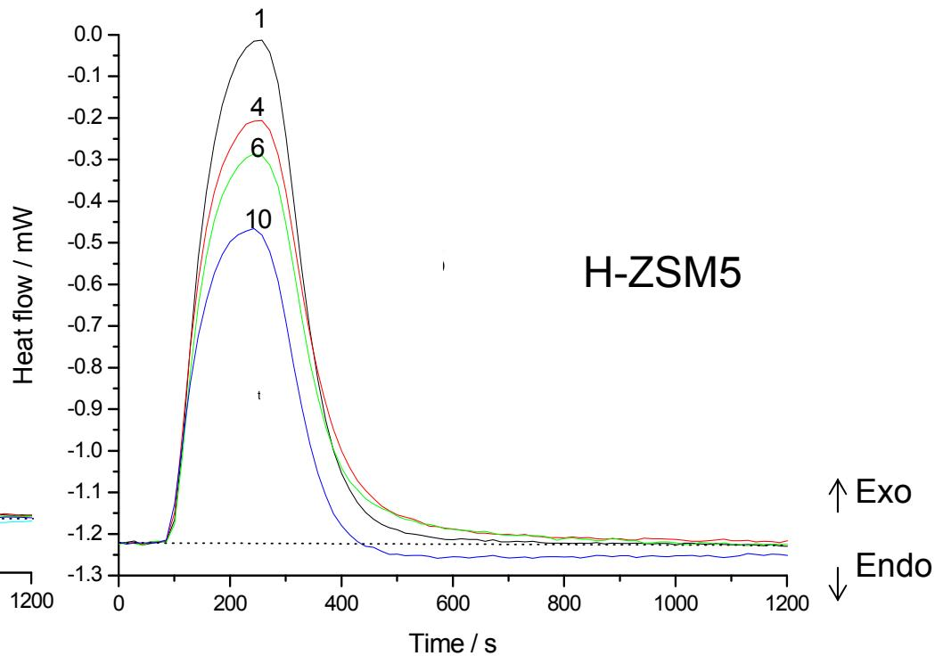
The shape of the calorimeter signal changes as the solid acid becomes progressively saturated
