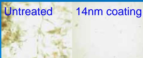
Microscopic examination of the fungal growth demonstrated production of aerial hyphae and spores on the untreated surface and only evidence of quiescent spores with limited or no hyphal growth on the 14nm coated surface.
