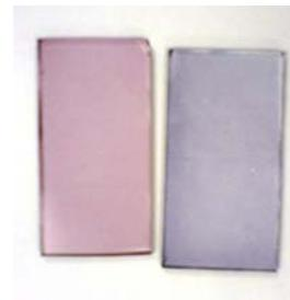
Spray deposition of gold nanoparticles incorporated into  $\text{TiO}_2$  matrix before (left) and after (right) annealing at  $400^\circ\text{C}$
