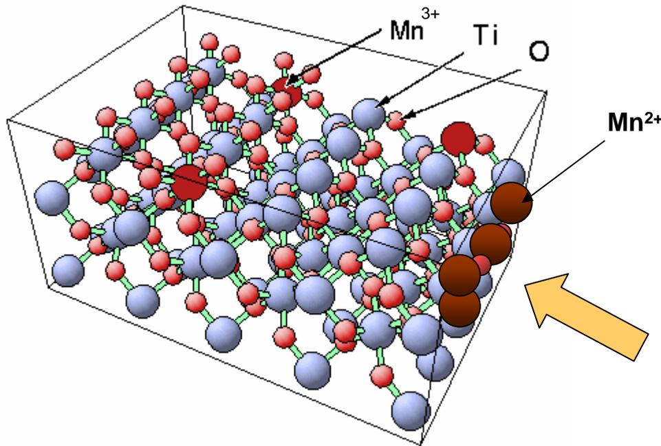
Rutile  $P4_2/mnm$  Titanium Oxide lattice
