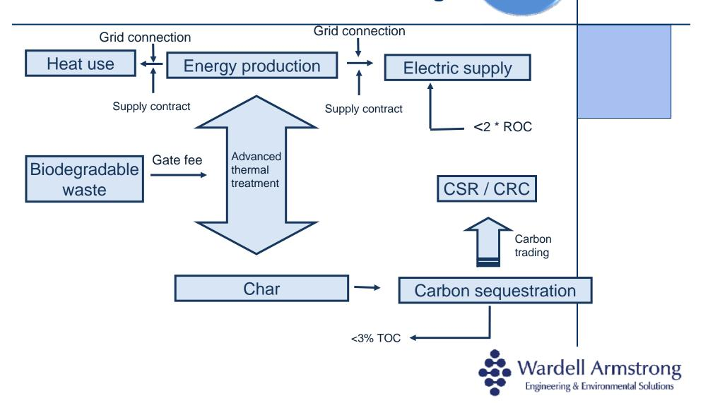
**Potential routes** using pyrolysis gasification
