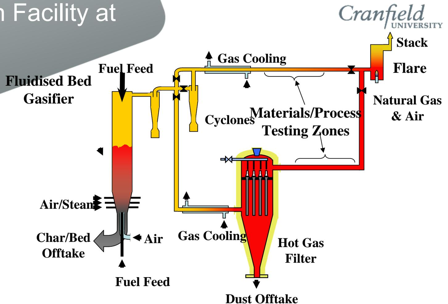
Spouted fluidised bed gasifier – 0.15m diameter
