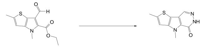
Initial conditions: Hydrazine hydrate, 2-ethoxyethanol, reflux; 79% yield
