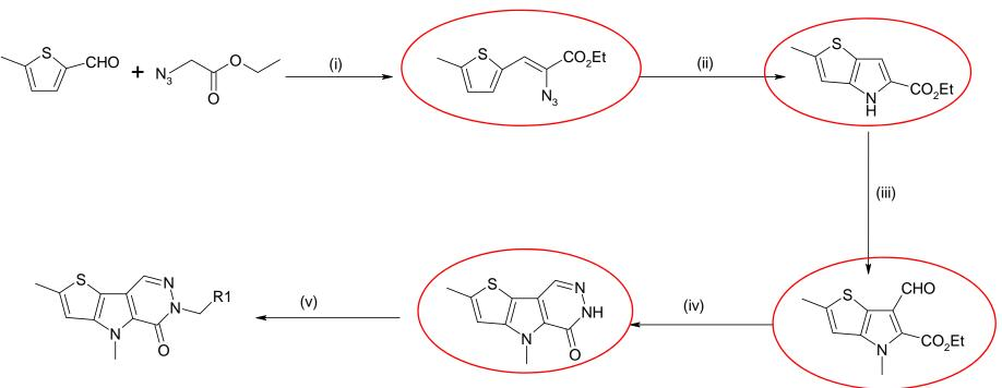
Conditions and reagents: (i) Na, EtOH, 0°C; (ii) xylene, reflux; (iii) (a) POCI<sub>3</sub>, DMF, 60°C, (b) MeI, K<sub>2</sub>CO<sub>3</sub>, DMF; (iv) 2-Ethoxyethanol, hydrazine, reflux; (v) alkyl bromide, KO<sup>t</sup>Bu, DMF, r.t.
