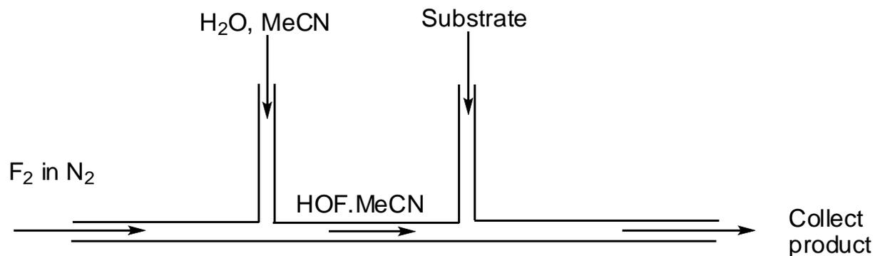
Gas/liquid – liquid/liquid sequential flow reaction
