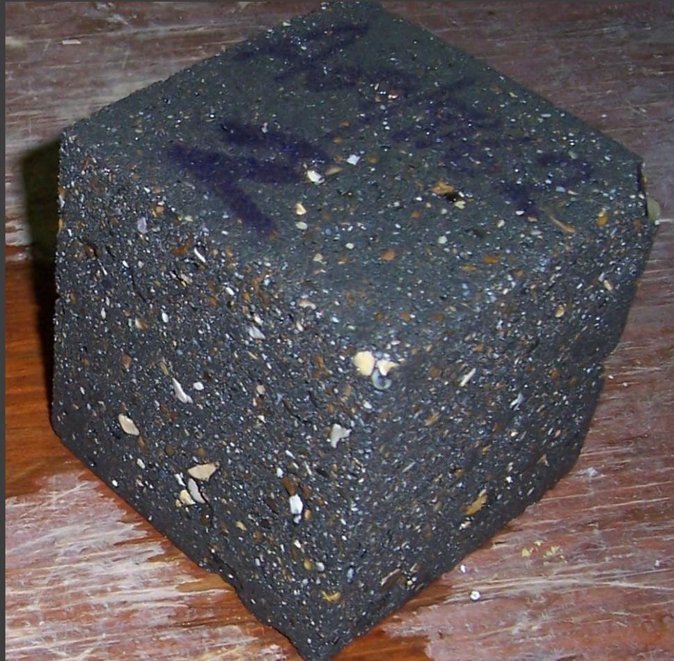
PC/pfa control: 15 months in Class 4a sulfate solution
