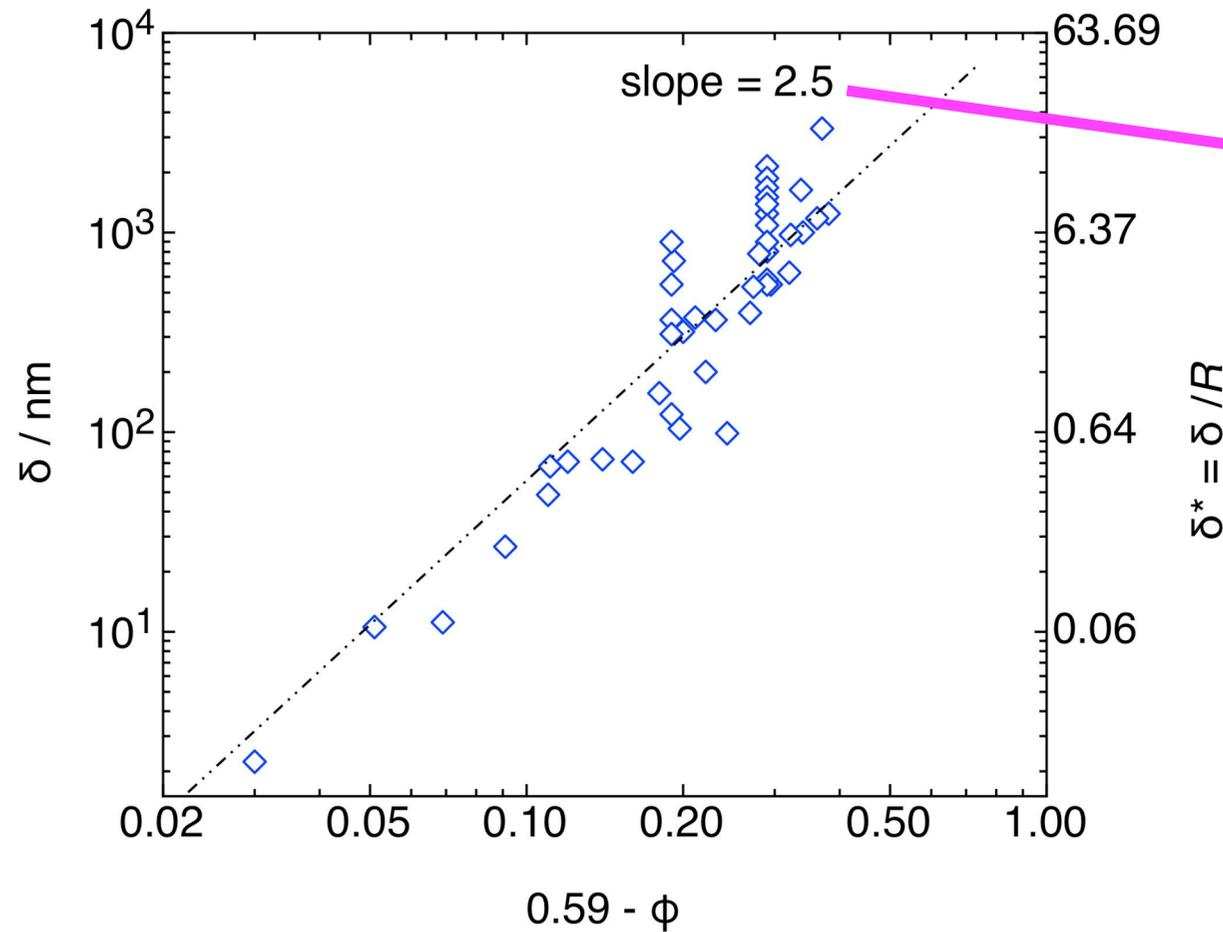
**Fig.1** Apparent slip layer thickness  $\delta$  (left) and scaled thickness  $\delta/R$  (right) versus volume-fraction for depletion flocculated latex of mean particle radius  $R = 157\text{nm}$ . Data taken from Buscall *et al.* (1993). A concentration exponent of ca. 2.5 is indicated.
