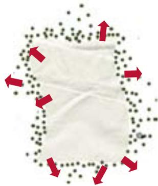
Zone of inhibition in Agar diffusion tests
