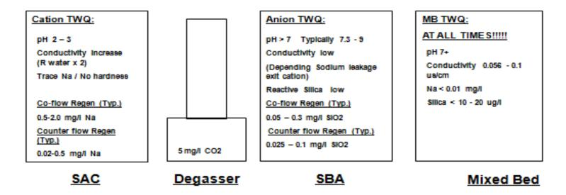
Raw Water Conductivity and pH (and temp variations if heated) Intermediate Stage Quality with regard to pH / Conductivity / Na / Silica
