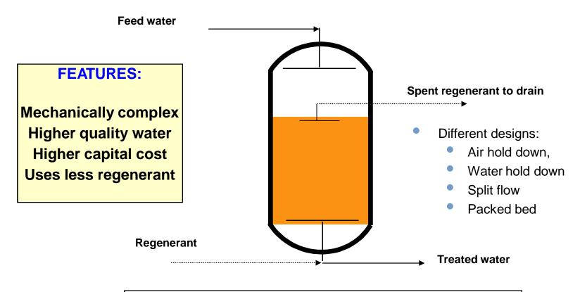
NOTE: Counter-flow regeneration may be difficult when water has elevated suspended solids
