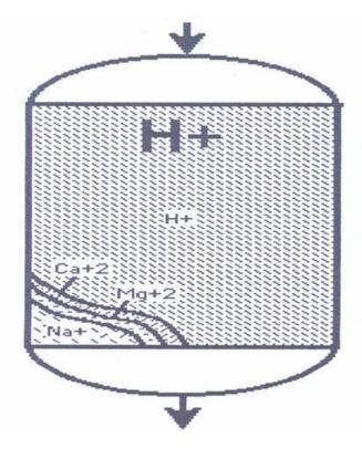
Trace cations at bottom of regenerated resin bed results in leakage
