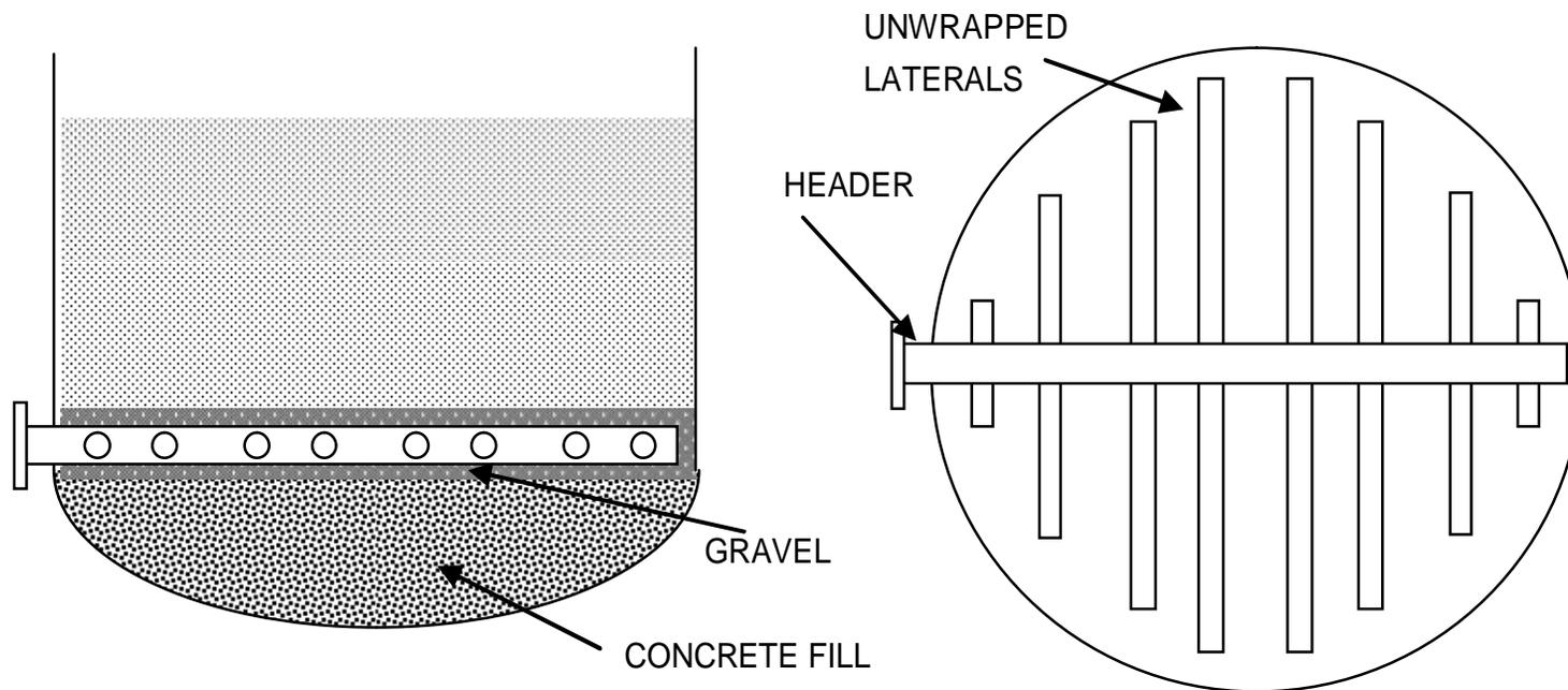
*Concrete fill with unwrapped laterals and gravel
